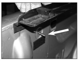
3. Align and push bolt through hole on inside wall of box and hold there for next step.
