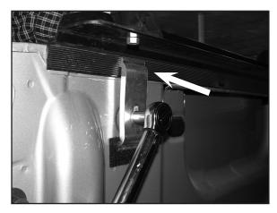
Adjust side rail height to clear tailgate as specified in owner's manual and hold it there. Push clamp up under side rail and tighten bolt. Torque this bolt to 18 ft. lbs. Repeat for opposite side.
