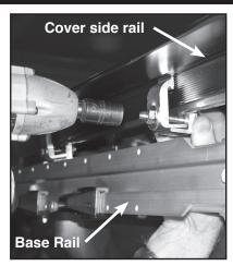
2. Hold clamp up as shown. Make sure clamp is located where two layers of sheet metal are present and tighten. Locate each clamp as shown on diagram above, and tighten.
