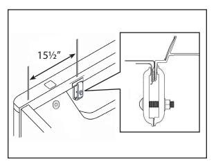
ALTERNATE LOCATION OF LONG CLAMP – only if stake pocket is not available. Even if stake pocket is utilized with an accessory, remove it and check for space. Usually the long clamp will install down in the pocket and still allow the accessory to be remounted.
