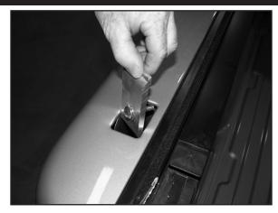
2. At top of rear stake pocket, lower back half of long clamp with carriage bolt down into pocket.
