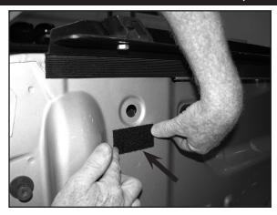
After short clamps are installed as shown on page 1, at rear of box under large hole in line with stake pocket, clean area and apply self adhesive protective strip.
