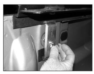
4. Place other half of clamp over bolt and turn nut on finger tight.
