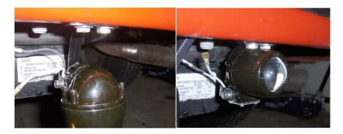
• With The Hardware Installed - Flip The Projector Up and Tighten The Hinge.
