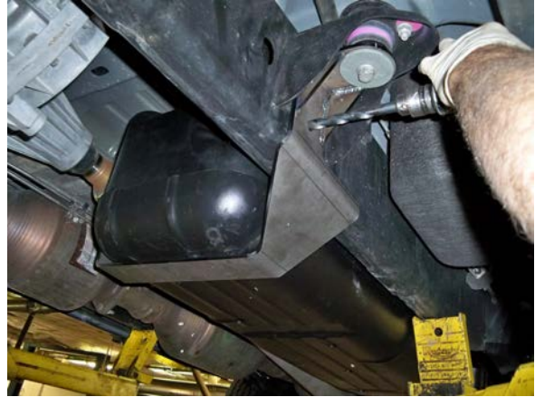
(Fig. 5) On 7030210 (Crew Cab, Short Bed) tanks only, bolt the Front Support to the nearest cab mount (as shown above), then use a 1/2" drill bit to drill through the support hole and through the vehicle's frame. Bolt the support to the frame using the bolt and hardware provided.
