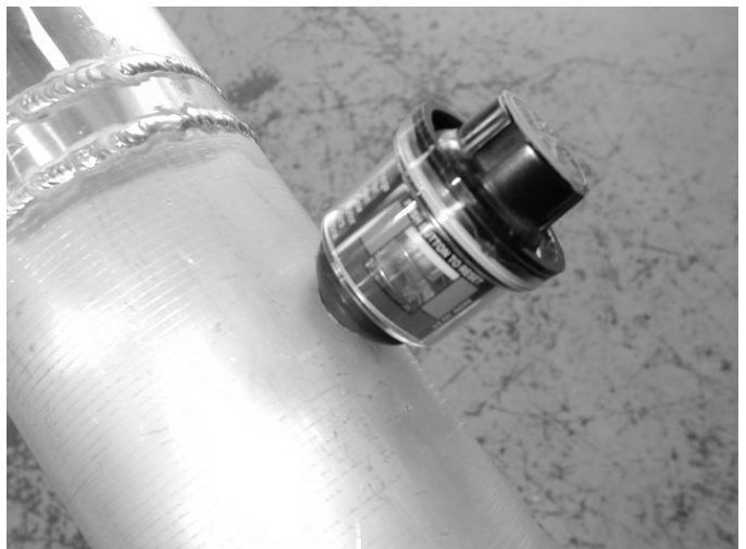
c) Insert the filter status meter and grommet into the hole in the inlet pipe.
