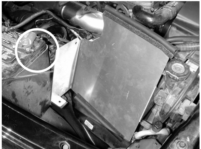
g) Place the heat shield in the engine bay as shown.
