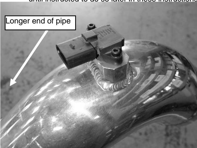
b) Install the IAT sensor in the Brute Force Inlet Pipe using the supplied screws. Make sure the electrical plug is pointed towards the longer section of piping.
