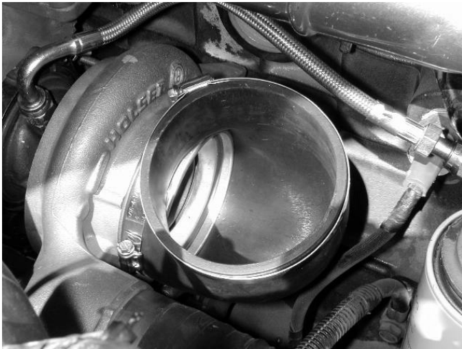
d) Install the short arm of the elbow onto the turbo inlet with the supplied hose clamp. Do not tighten the clamp.
