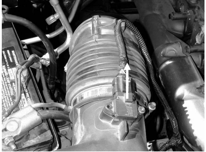
b) Unplug the Inlet Air Temperature (IAT) sensor.
