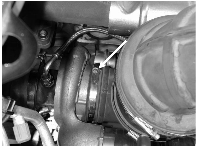
d) Loosen the hose clamp at the turbo inlet and pull the hose off of the turbo.
