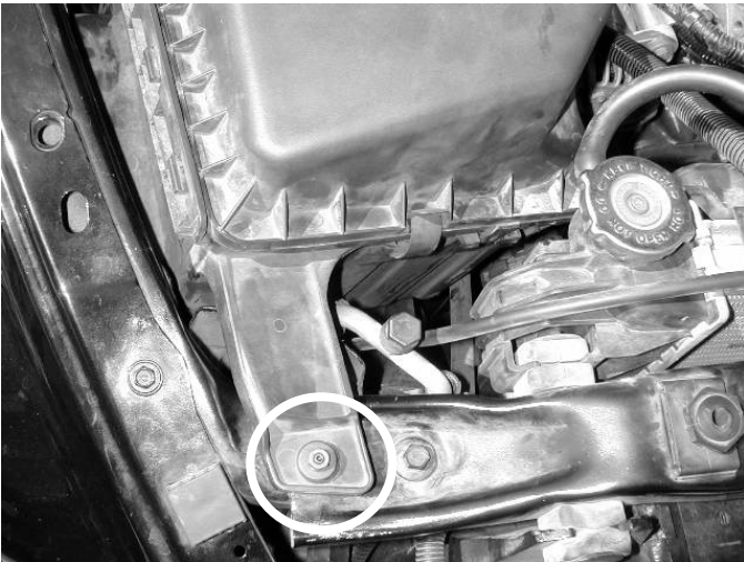
c) Remove the nut securing the front tab of the air box.
