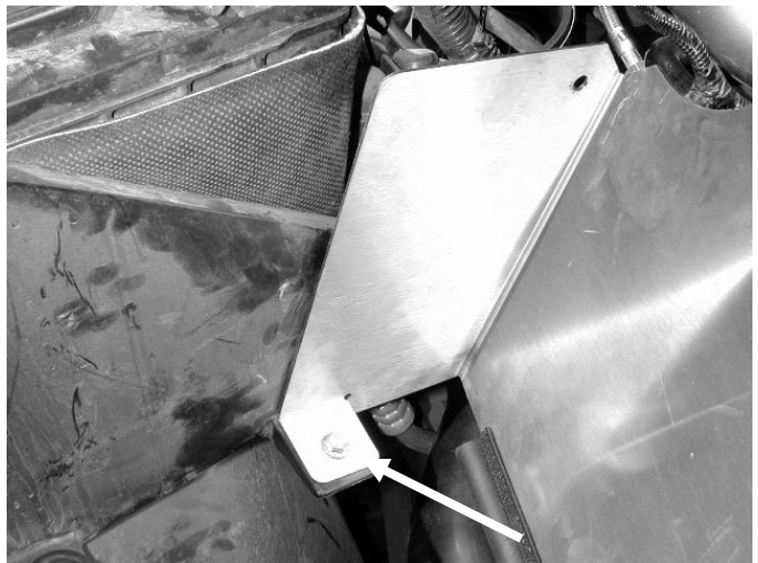
i) Secure the lower tab with the supplied bolt, washer and lock nut. The washer and lock nut should be installed from the bottom, underneath the plastic tab.
