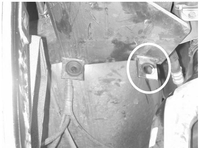
h) Remove the grommet from the inner air box mounting tab.
