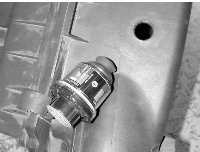
g) Extract the filter status meter and its grommet from the air box.
