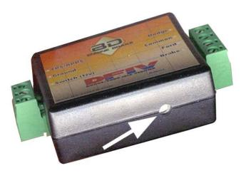
screwdriver, turn the small adjusting screw in the DFIV Module counterclockwise or clockwise until the test light JUST turns on.
