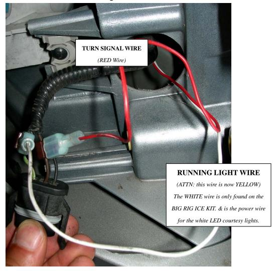
**5.** Now you are ready to test the bar by turning on your headlights and activating your hazard lights to confirmthat the bar illuminates properly and gets brighter as the hazard lights blink. Once you have confirmed that everything is working as it should, complete the assembly of the drivers side and begin the installation of the remaining L.E.D. bar on the passenger side of the truck by repeating everything you have done to the drivers side.
