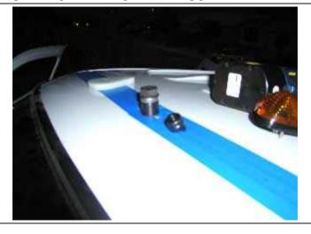
Then use a Knock Out (7/8") tool to make the center holes for the lights. The outer holes for the studs are drilled to 1/4" to provide some fudge room. Keep the shop vac hose handy to vacuum the shavings as you go along.
