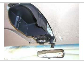
Be patient with this step. Gently tug on the plastic cover for the overhead console to pop it loose. It sounds like it's breaking apart, but it's just the clips coming loose. Leave the inner portion attached. You can work around it!
