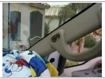
First thing you need to do is cover your dash to keep shavings and stuff from falling into your interior. You have to take down the front of your headliner to access the area for the cab lights and to remove and install the harness. Remove the plugs on the handle on the passenger side and then remove the (4) bolts holding the handle on.... required a 5/16" socket.
